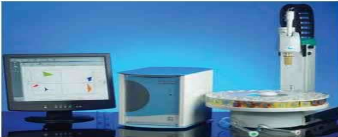
FIGURE 4.4 Electronic tongue to assist in formulation development. (Courtesy of Alpha MOS.)
